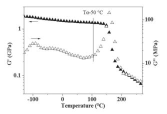
**Fig. 5.** Evolution of the conservative  $G'(\blacktriangle)$  and dissipative  $G''(\triangle)$  modulus of PEKK versus temperature.
