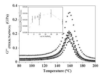
**Fig. 7.** Imaginary part of the shear modulus (■) versus temperature of PEKK and PEKK/NaNbO<sub>3</sub>: (■) PEKK, (○) PEKK/NaNbO<sub>3</sub> 4 vol%, (▲) PEKK/NaNbO<sub>3</sub> 6 vol%, (▽) PEKK/NaNbO<sub>3</sub> 9 vol%, (♦) PEKK/NaNbO<sub>3</sub> 10 vol%, (⊲) PEKK/NaNbO<sub>3</sub> 11 vol%, (►) PEKK/NaNbO<sub>3</sub> 20 vol%, (★) PEKK/NaNbO<sub>3</sub> 30 vol%. In the inset: specific energy loss normalized by the matrix fraction versus vol%.
