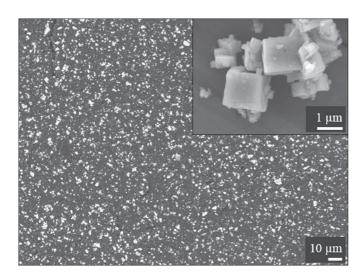
**Fig. 1.** SEM image of PEKK/NaNbO<sub>3</sub> micro cut with a volume fraction of 20% (scale bar: 10 μm). In the insert: NaNbO<sub>3</sub> particles (scale bar: 1 μm).
