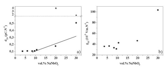
Fig. 8. Evolution of the piezoelectric coefficient  $d_{33}$  ( $\blacksquare$ ) fitted with the Furukawa's model (solid line) a) and the piezoelectric voltage constant  $g_{33}$  ( $\blacksquare$ ) b) of PEKK/NaNbO<sub>3</sub> versus NaNbO<sub>3</sub> vol%. ( $\bigstar$ ) corresponds to PVDF/NaNbO<sub>3</sub> and ( $\blacktriangle$ ) PZT/PEEK nanocomposites [5].
