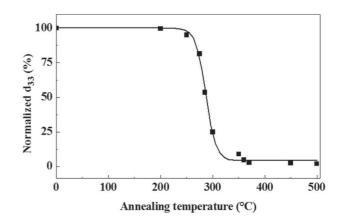
Fig. 2.  $d_{33}$  evolution of NaNbO<sub>3</sub> disk versus annealing temperature. The line is drawn as a guide to the eyes.
