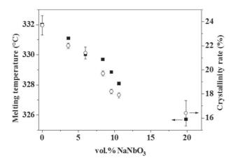
**Fig. 4.** Melting temperature (■) and crystallinity ratio (○) versus NaNbO<sub>3</sub> vol% for PEKK/NaNbO<sub>3</sub> nanocomposites during the 2nd run.
