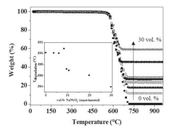
**Fig. 3.** TGA thermogram of PEKK and PEKK/NaNbO<sub>3</sub>: (■) PEKK, (○) PEKK/NaNbO<sub>3</sub> 4 vol%, (▲) PEKK/NaNbO<sub>3</sub> 6 vol%, (▽) PEKK/NaNbO<sub>3</sub> 9 vol%, (♦) PEKK/NaNbO<sub>3</sub> 10 vol%, (⊲) PEKK/NaNbO<sub>3</sub> 11 vol%, (►) PEKK/NaNbO<sub>3</sub> 20 vol%, (★) PEKK/NaNbO<sub>3</sub> 30 vol%. In the inset: evolution of the degradation temperature versus the experimental vol% of NaNbO<sub>3</sub>.
