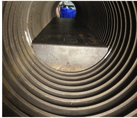
Figure 3: Interior view of the stiffened cylindrical shell with the non-axisymmetric internal frame.
