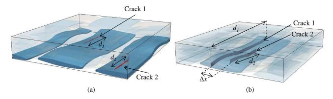
Figure 9: Damaged cell containing two cracks (a) in two different yarns and (b) in the same yarn.
