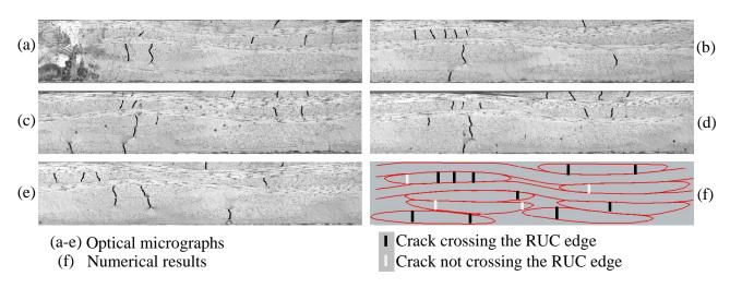
Figure 18: Comparison between crack locations (a-e) observed experimentally on the edge of the specimen and (f) obtained numerically for a crack density  $\rho_c = 0.18 \text{ mm}^{-1}$ .
