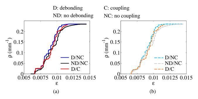
Figure 11: Comparison of damage growth obtained with or without coupling between close cracks using (a) or not (b) the energy surplus for further crack propagation.
