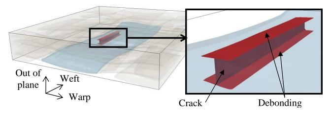
Figure 4: Discrete damage modeling in the representative unit cell of the composite. Example of an intra-yarn crack with debonding at the crack front.
