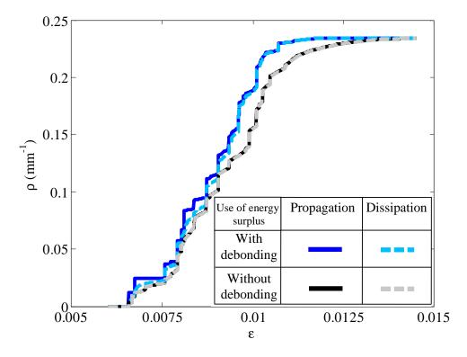
Figure 8: Crack density as a function of strain with or without debonding using the energy surplus of the unstable phase for further crack propagation, or not (dissipation).
