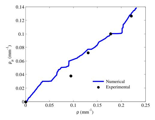
Figure 14: Relationship between debond  $(\rho_{\mu})$  and crack  $(\rho)$  densities obtained numerically (in blue) and experimentally (in black).
