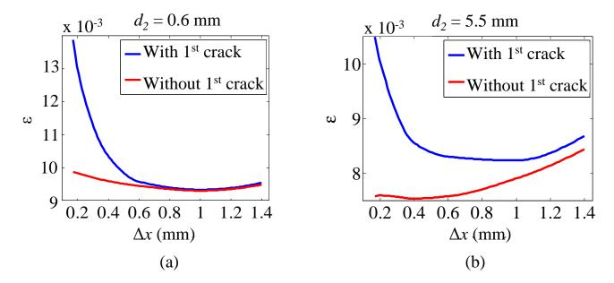
Figure 10: Initiation strain of a second crack (a) 0.6 mm and (b) 5.5 mm in length as a function of the distance  $\Delta x$  along the warp direction from another crack (in blue) or without the presence of other cracks (in red).
