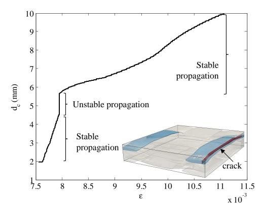
Figure 5: Crack length as a function of the macroscopic strain. Crack propagation is stable for  $d_c < 4.6$  mm and  $d_c > 5.7$  mm, and unstable for  $4.6 < d_c < 5.7$  mm.
