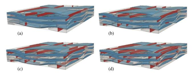
Figure 15: Damage in the cell predicted for the crack density levels measured experimentally: (a)  $\rho_c = 0.09~\mathrm{mm}^{-1}$ , (b)  $\rho_c = 0.13~\mathrm{mm}^{-1}$ , (c)  $\rho_c = 0.18~\mathrm{mm}^{-1}$ , (d)  $\rho_c = 0.22~\mathrm{mm}^{-1}$ .
