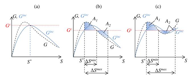
Figure 3: Incremental and differential energy release rates as functions of the crack surface in the case of (a) stable and (b-c) unstable propagations of a crack.
