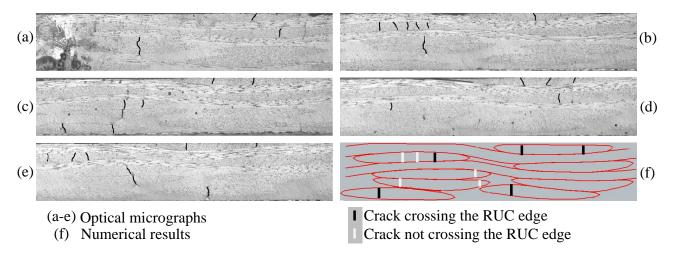
Figure 16: Comparison between crack locations (a-e) observed experimentally on the edge of the specimen and (f) obtained numerically for a crack density  $\rho_c = 0.09 \text{ mm}^{-1}$ .
