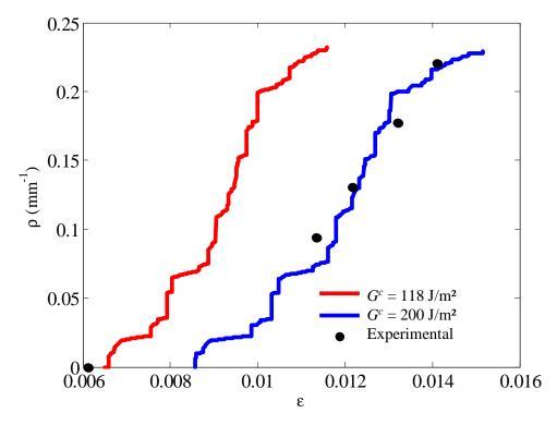
Figure 12: Crack density as a function of strain obtained when  $G^c = 118 \text{ J/m}^2$  (in red),  $G^c = 200 \text{ J/m}^2$  (in blue), and observed experimentally (in black).
