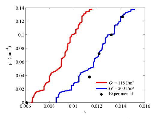
Figure 13: Debonding density as a function of strain obtained when  $G^c = 118 \text{ J/m}^2$  (in red),  $G^c = 200 \text{ J/m}^2$  (in blue), and observed experimentally (in black).
