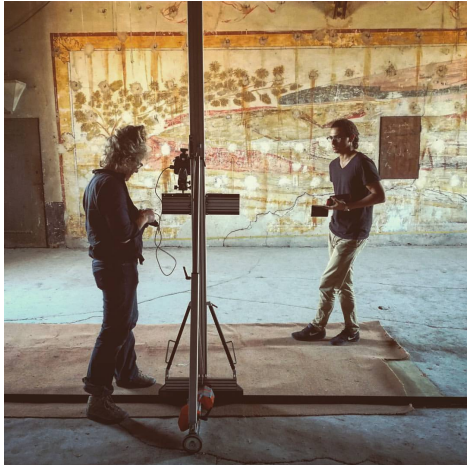
Figure 6: In-situ view of the data acquisition set-up during Anamorphosis case-study survey
