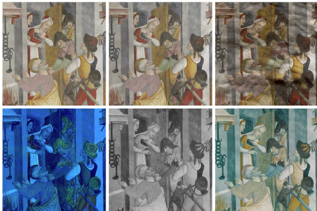
Figure 1: Example of TP documentation on The Denial of Saint-Peter fresco from the case-study of Notre-Dame des Fontaines chapel ; respectively VIS, semi-RAK (from right), RAK (from down), UVf, IR and IRf
