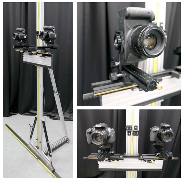
Figure 5: Views of the mechanical structure ; complete system on the traveling rail (left), close-up on the double micrometric plates (X and Z) with a camera vertically mounted (upper-right) and close-up on Y translation plate with two cameras in horizontal position (bottom-right)
