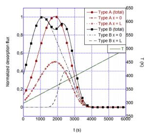
Fig. 4 – Simulated normalized TDS spectra for Type A and Type B charging subjected to 30 min of aging at 298 K between charging and TDS ( $\phi = 2 \text{ K min}^{-1}$ ). All desorption flux (x = 0 and x = L) are shown.
