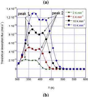
Fig. 5 – Simulated theoretical desorption spectra for  $\phi$  ranging from 2 to 15 K min<sup>-1</sup> for charging (a) Type A and (b) Type B. Simulations incorporated a 30 min aging period between charging and TDS analysis.
