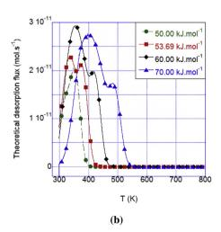
Fig. 11 – Effect of activation energy: (a)  $E_k$  and (b)  $E_p$ , on simulated TDS spectra ( $\phi = 2$  K min<sup>-1</sup>) for aged samples of charging Type B.
