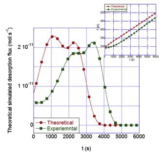
Fig. 8 – Simulated TDS spectrum for a linear theoretical T ramp ( $\phi=2$  K min<sup>-1</sup>) as compared to an experimental T ramp ( $\phi=2$  K min<sup>-1</sup>). The graphic insert shows the linear T ramp as compared to an experimental acquired T ramp: y-axis: T (K), x-axis: t (s).
