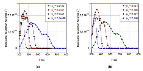
Fig. 9 – Effect of pre-exponential factor: (a)  $k_0$  and (b)  $p_0$ , on simulated TDS spectra ( $\phi = 2$  K min<sup>-1</sup>) for aged (30 min at 298 K) samples of charging Type B.
