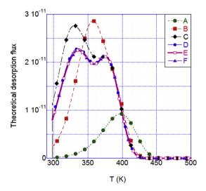
Fig. 10 – Influence of  $k_0/p_0$  with a constant ratio ( $k_0/p_0=1.25$ ) on a simulated TDS spectrum ( $\phi=2$  K min<sup>-1</sup>), see Table 4 for the corresponding  $k_0$  and  $p_0$  simulation values (A–F). The samples were Type B charged (Table 3) and aged 30 min at 298 K.
