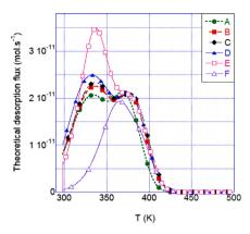
Fig. 12 – Influence of  $E_k$  and  $E_p$  when  $E_b$  is held constant at 48 kJ mol<sup>-1</sup> on simulated TDS spectra, see Table 5 for the corresponding  $E_k$  and  $E_p$  simulation values (A–F). The samples were supposed charged using Type B conditions (Table 3) and aged 30 min at 298 K.
