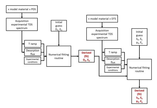
Fig. 13 — Logic diagram of proposed analysis method coupling experimental results with a numerical analysis fitting technique in order to derive both the diffusion and trapping/detrapping parameters.
