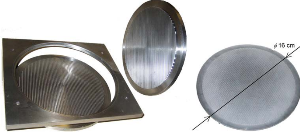
Fig. 3. Photograph of the mould used to process the crenellated membranes (left) and photograph of a resulting crenellated plate (right).
