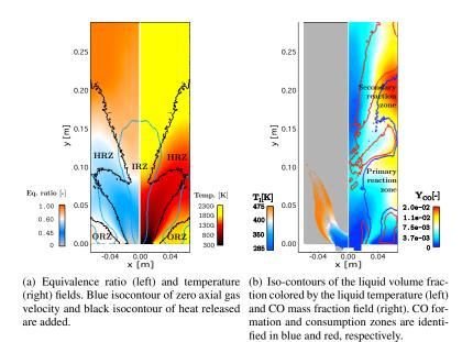
Fig. 7: Time-averaged flame structure.
