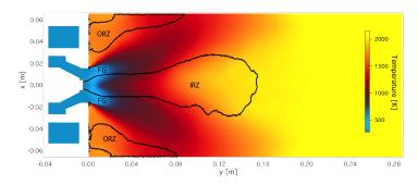
Fig. 2: Mean gas temperature distribution. In order to localize the recirculation zones black isocontour of zero axial gas velocity is added.
