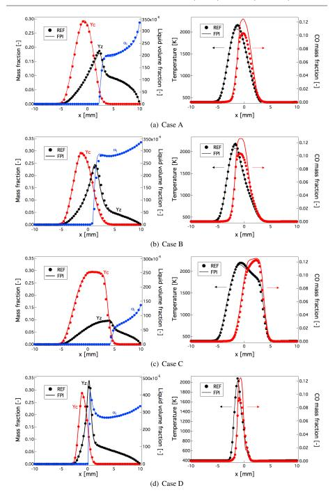
Fig. 17: Counterflow laminar spray flames of Table 1 (A-D from top to bottom). Comparison between the reference detailed model (symbols) and the tabulated description (line): axial profiles of mixture fraction, progress variable and liquid volume fraction (left), temperature and CO mass fraction (right).
