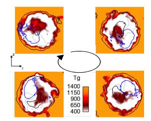
Fig. 9: Pressure, liquid volume fraction and mass transfer iso-contours are represented at four instants of one period of the PVC on the first measurement plane (x=8 mm), for p=0.995 MPa (blue),  $\alpha_l=2.\cdot 10^{-4}$  (grey) and  $\dot{m}=0.05$  kg.m $^{-3}$ .s $^{-1}$  (black) respectively. For  $\dot{m}$ , the maximum values are reached outside the external contour and inside the internal contour. The colormap denotes the instantaneous gas temperature distribution saturated at 1400 K.
