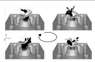
Fig. 8: Instantaneous pressure iso-surface in black ( $P=0.10\,$  MPa) and liquid volume fraction iso-surface in white ( $\alpha_l=2.4\cdot 10^{-4}$ ). Four instantaneous solutions are considered at equidistant times for one period of the PVC.
