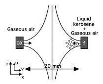
Fig. 16: Schematic of a laminar counterflow spray flame.
