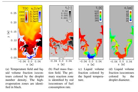
Fig. 5: Characterization of the primary reaction zone.
