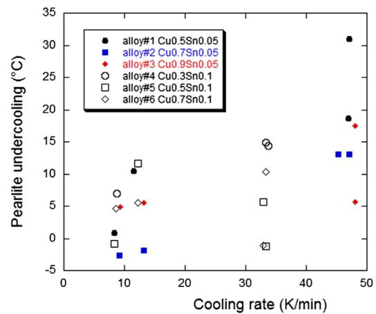
5 Pearlite undercooling with respect to the calculated  $T_p$  temperature for the start of austenite transformation to pearlite vs. the cooling rate  $V_r$  (see text)
