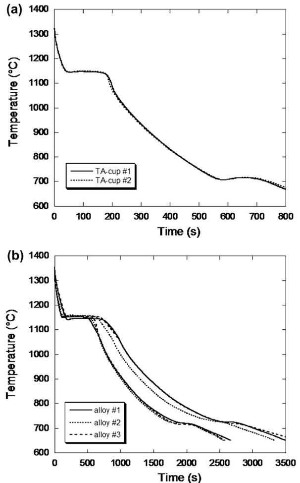
**1** a Comparison of the two TA-cup thermal records for alloy #2; b records from the two keel blocks for all three alloys of the Sn0.05 series (first and second keel blocks are differentiated by the overall cooling time, see text)
