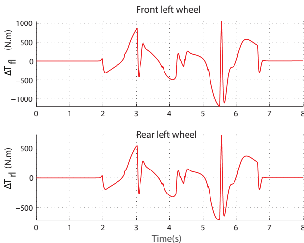
Fig. 6. Driving/braking torques applied by the controller to the left wheels.
