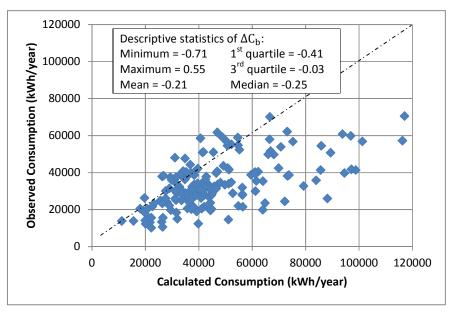
**Figure 1.** Observed and calculated consumption (all end-uses) before retrofitting of 167 individual houses. *Dotted line is the diagonal showing equivalence between observed and calculated consumptions.*
