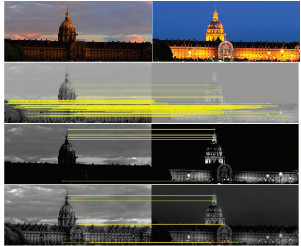
Fig. 7: Repeated Keypoints. Row I: 2 HDR images from Invalides scene taken at different day-time. HDR images are displayed after log scaling[14]. Row II: the repeated keypoints using our proposed AdTMO (66 repeated keypoints out of strongest 200 keypoints). Row III: the repeated keypoints using Reinhard TMO (7 repeated keypoints out of strongest 200 keypoints). Row IV: the repeated keypoints using MantiukTMO (5 repeated keypoints out of strongest 200 keypoints).
