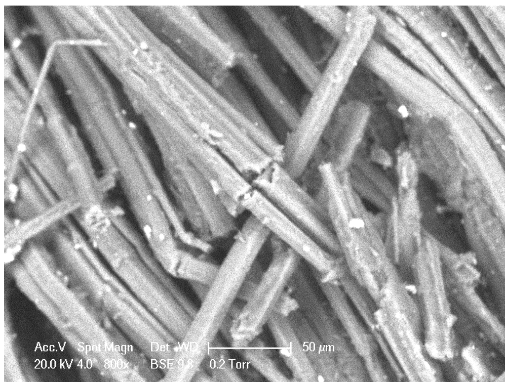
Figure 7: Cracks, twisting, and warping in fibers.
