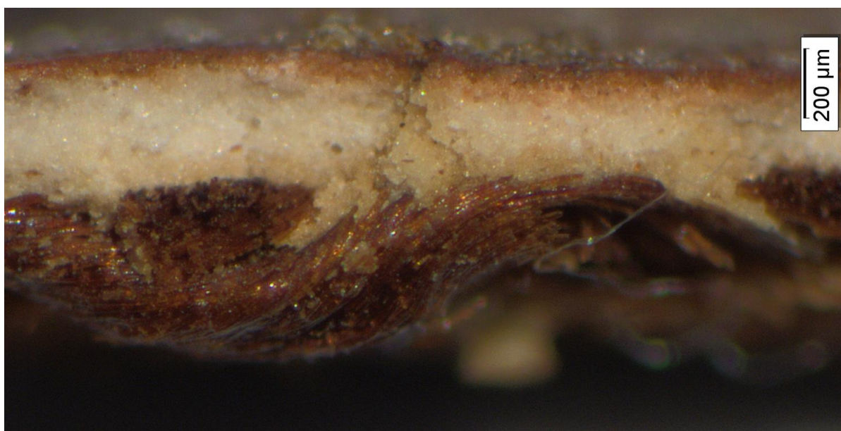
Figure 9: Cross section of the ground layer and pigments.
