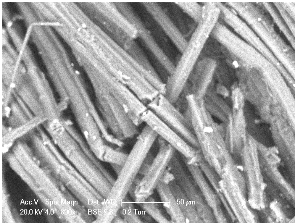
Figure 7: Cracks, twisting, and warping in fibers.
