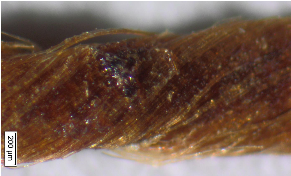
Figure 5: Linen fibers through the optical microscope, showing hardening of the linen fibers.
