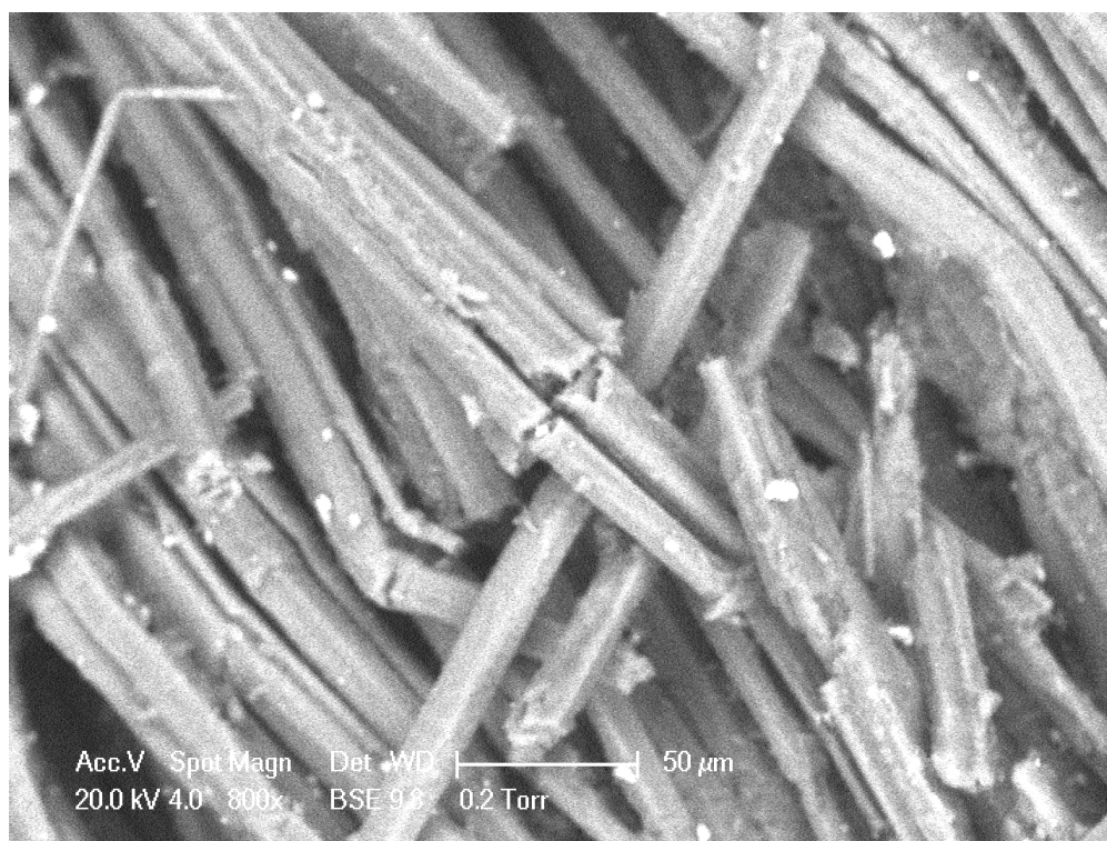
Figure 7: Cracks, twisting, and warping in fibers.
