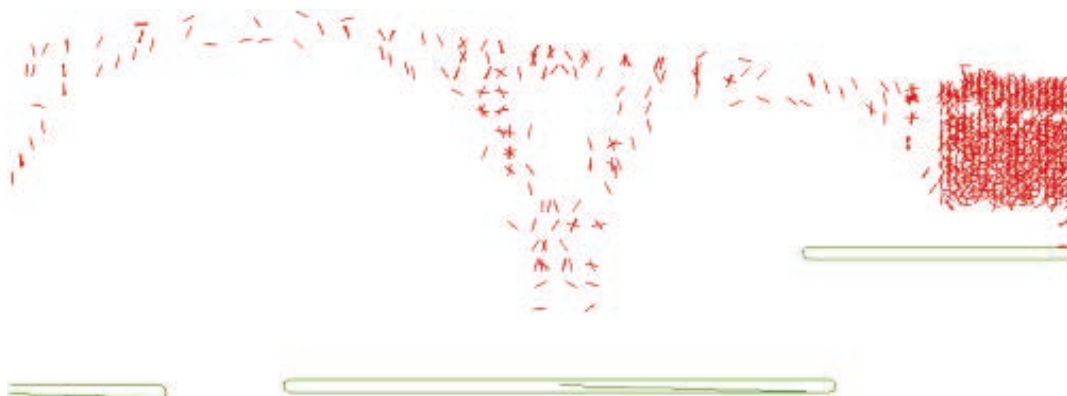
Figure 27. Weak contacts: normal reaction less than the average value.
