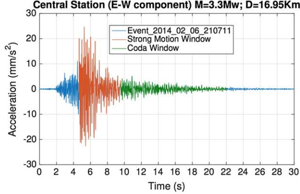
Figure 7. Strong motion window used for estimating coherency of earthquake ground motions. [Colour figure can be viewed at [wileyonlinelibrary.com](http://wileyonlinelibrary.com)]
