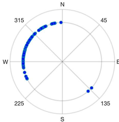
Figure 10. Distribution of angle  $\phi$  representing the directions of plane-wave propagations. The center of circle corresponds to the station array. [Colour figure can be viewed at [wileyonlinelibrary.com](http://wileyonlinelibrary.com)]
