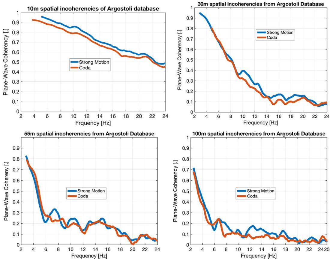
Figure 15. Comparison between coherencies estimated from strong motion windows and from coda parts of signals for 10, 30, 55 and 100 m of separations. [Colour figure can be viewed at [wileyonlinelibrary.com](http://wileyonlinelibrary.com)]
