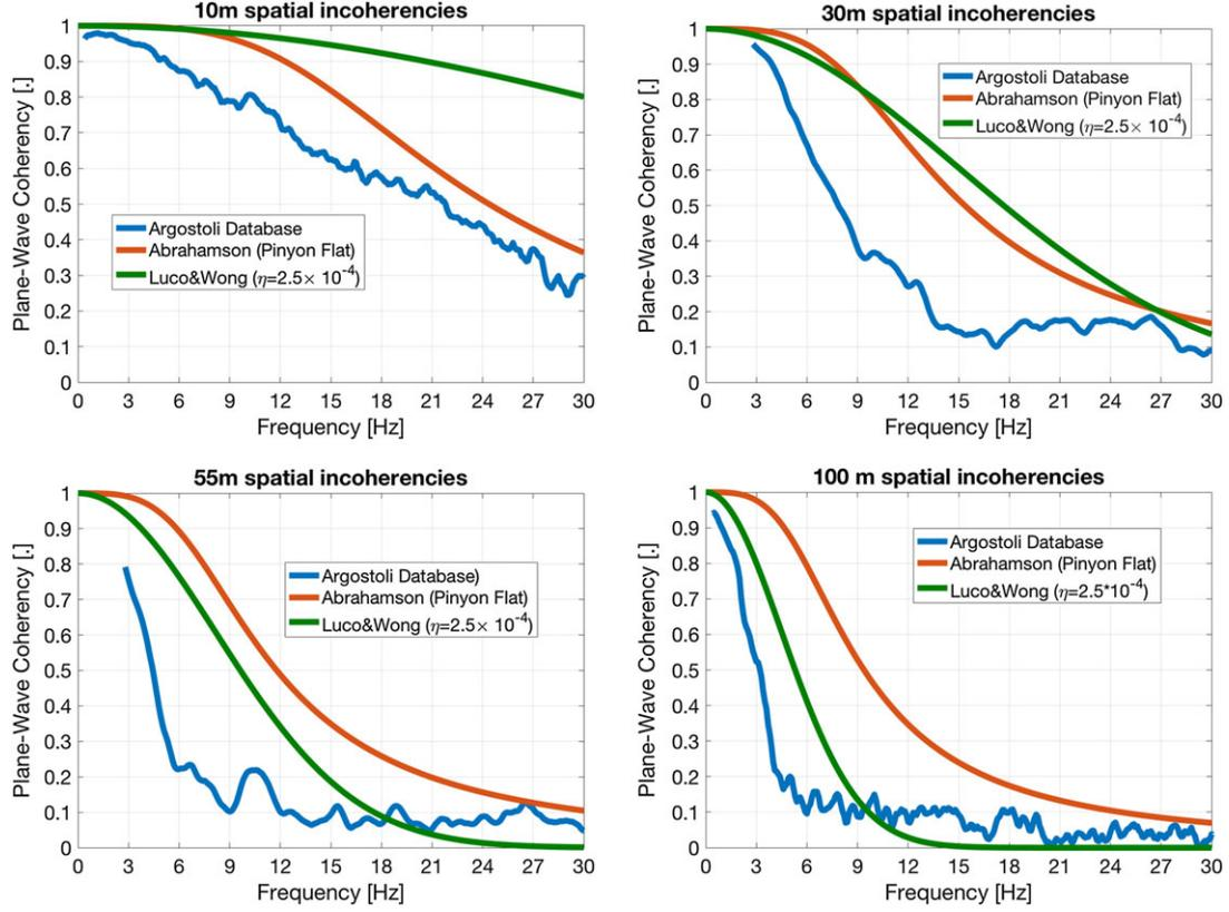
Figure 19. Comparison between coherencies estimated from Argostoli database and existing coherency models for 10, 30, 55 and 100 m of separations. [Colour figure can be viewed at [wileyonlinelibrary.com](http://wileyonlinelibrary.com)]
