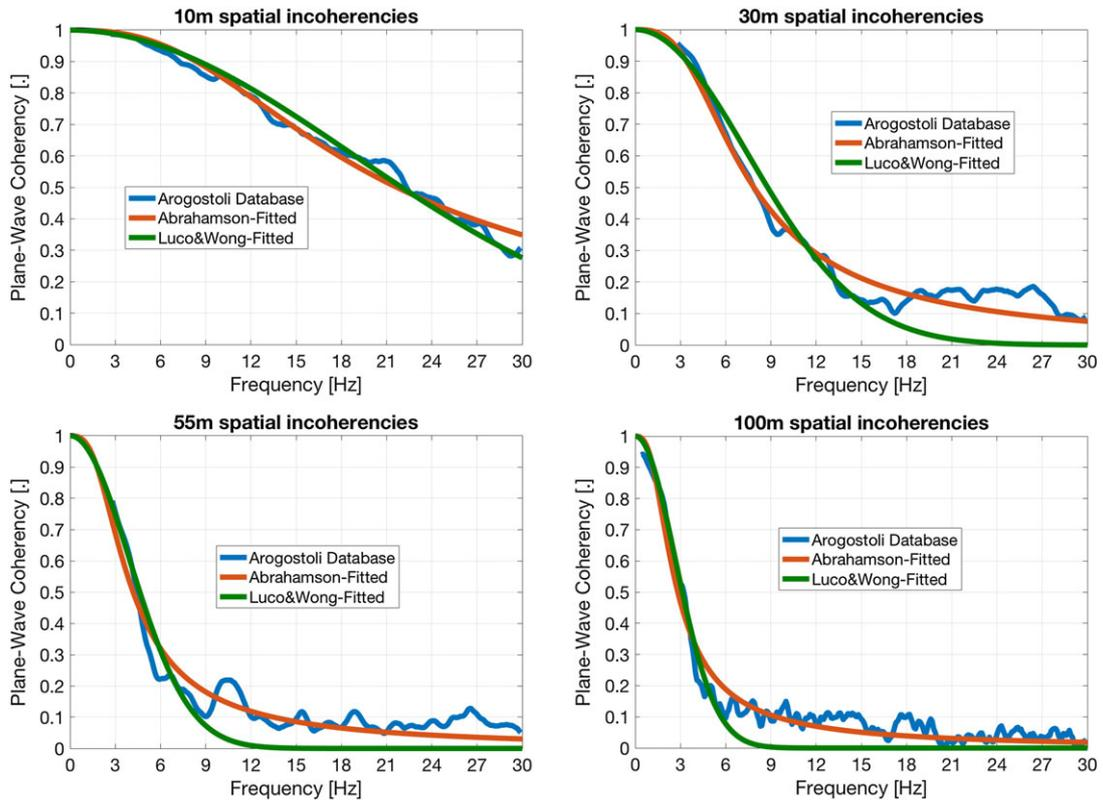
Figure 21. Comparison between coherencies estimated from Argostoli database and modified (fitted) coherency models for 10, 30, 55 and 100 m of separations. [Colour figure can be viewed at [wileyonlinelibrary.com](http://wileyonlinelibrary.com)]
