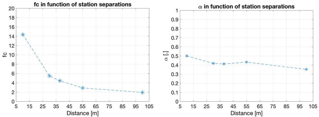
Figure 20. The values of parameters used for fitting existing coherency models with Argostoli coherencies. Left:  $f_c$  in function of station separations (for Abrahamson model). Right:  $\alpha$  in function of station separations (for the Model of Luco and Wong). [Colour figure can be viewed at [wileyonlinelibrary.com](http://wileyonlinelibrary.com)]
