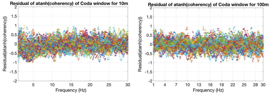
Figure 16. Residual of  $\tanh^{-1}(\text{coherencies})$  estimated from coda window of ground motion signals for 10 and 100 m of station separations. [Colour figure can be viewed at wileyonlinelibrary.com]
