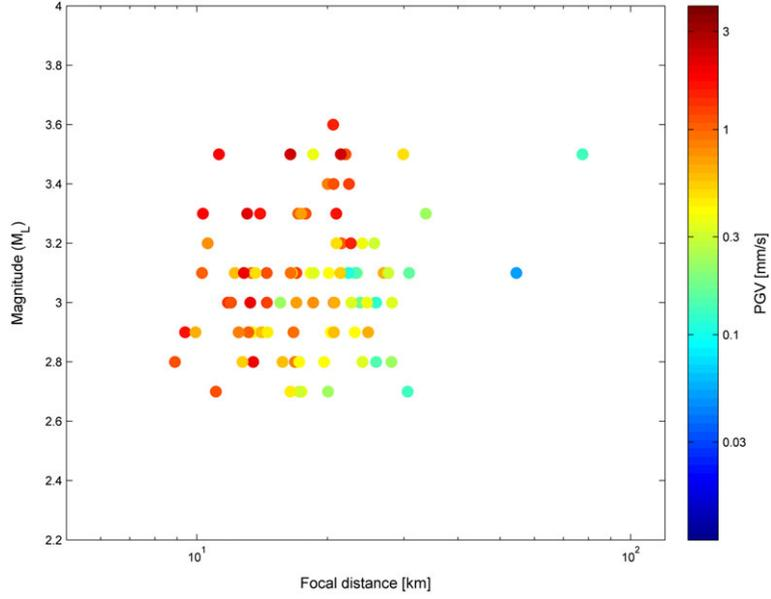
Figure 4. Distribution of selected earthquake in terms of epicentral distances ( $x$ -axis), magnitudes ( $y$ -axis) and peak ground velocity (color scale). [Colour figure can be viewed at [wileyonlinelibrary.com](http://wileyonlinelibrary.com)]
