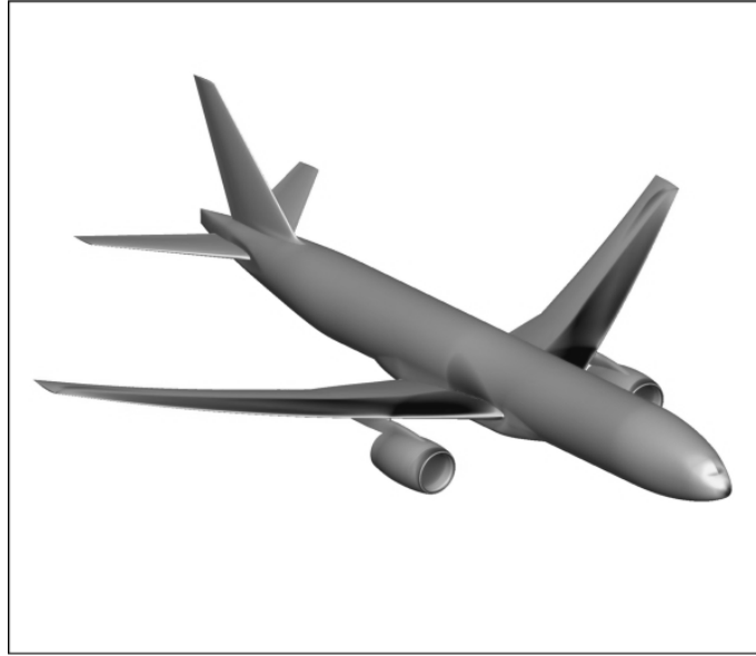
Fig. 24 Complete configuration; Ma = 0.85 , Re = 5 \times 10^6 , CL = 0.5 ; pressure field on suction side.
