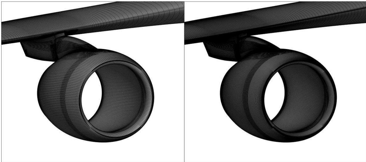
**Fig. 5 Nacelle-Pylon surface discretization; WBNP2 and WBNP5.**
