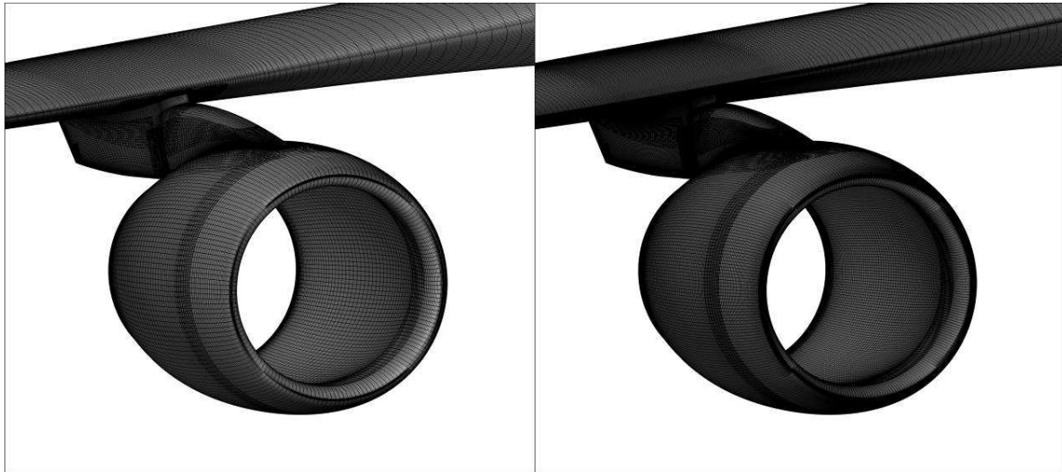
Fig. 5 Nacelle-Pylon surface discretization; WBNP2 and WBNP5.
