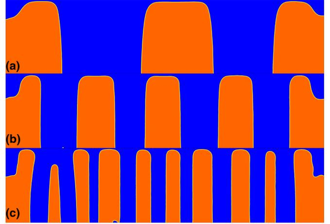
FIG. 4. Quasistationary band patterns in a two-layer system of silicon oil and Galden HT135 with densities and viscosities corresponding to experiment [18] (see text). Vibration characteristics are  $f = 30$  Hz: (a)  $a = 1.0$  mm; (b)  $a = 1.6$  mm; (c)  $a = 2.6$  mm.
