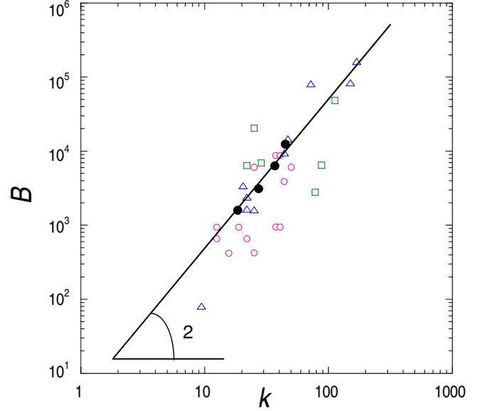
FIG. 11. Comparison of space data from Maxus 7 (triangles), Maxus 5 (open squares), and MiniTexus 5 (open circles) with the results of the linear stability analysis for viscous fluids [ $\nu_1 = \nu_2 \approx 5 \times 10^{-5}$ ] which can be approximated by a power law with exponent 2.
