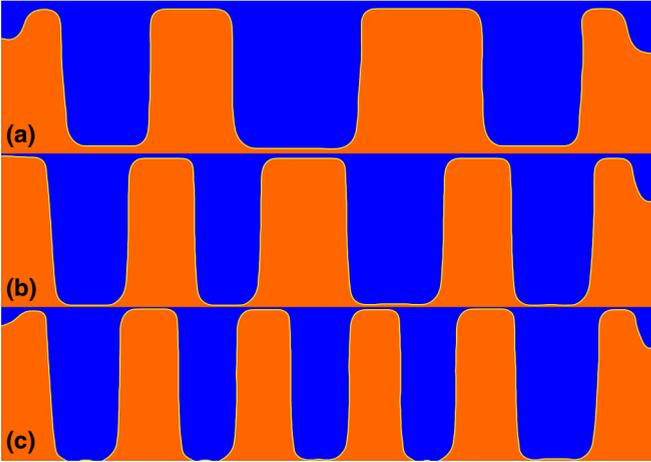
FIG. 5. Evolution of quasistationary band patterns with the decrease of dynamic viscosity for the vibration characteristics  $f = 30$  Hz and  $a = 1.8$  mm. Dynamic viscosities of both fluids are made equal (see text): (a)  $\eta = 0.2$  Pa.s; (b)  $\eta = 0.075$  Pa.s; (c)  $\eta = 0.04$  Pa.s.
