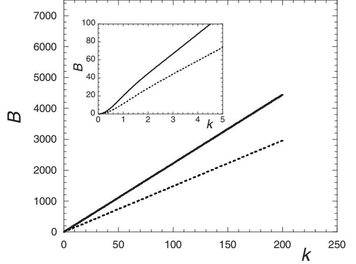
FIG. 2. Dependence of the dimensionless vibrational parameter  $B$  on the dimensionless wave number  $k$  for  $\rho = 1.07$ . Interrupted curve: Neutral perturbations with  $\sigma = 0$  in an inviscid fluid. Full curve: Perturbations with maximal growth rate in an inviscid fluid. Inset: Small  $k$  behavior.
