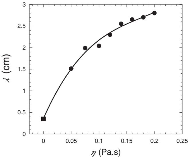
FIG. 6. Dependence of the pattern wavelength  $\lambda^*$  (cm) on dynamic viscosity  $\eta$  (Pa.s) for vibration characteristics  $f = 30$  Hz and  $a = 1.8$  mm. Filled circles are the results of DNS (see Fig. 5); the solid curve is a smoothing function. The full square is the value calculated from the analytical formula Eq. (28) obtained for inviscid fluids.
