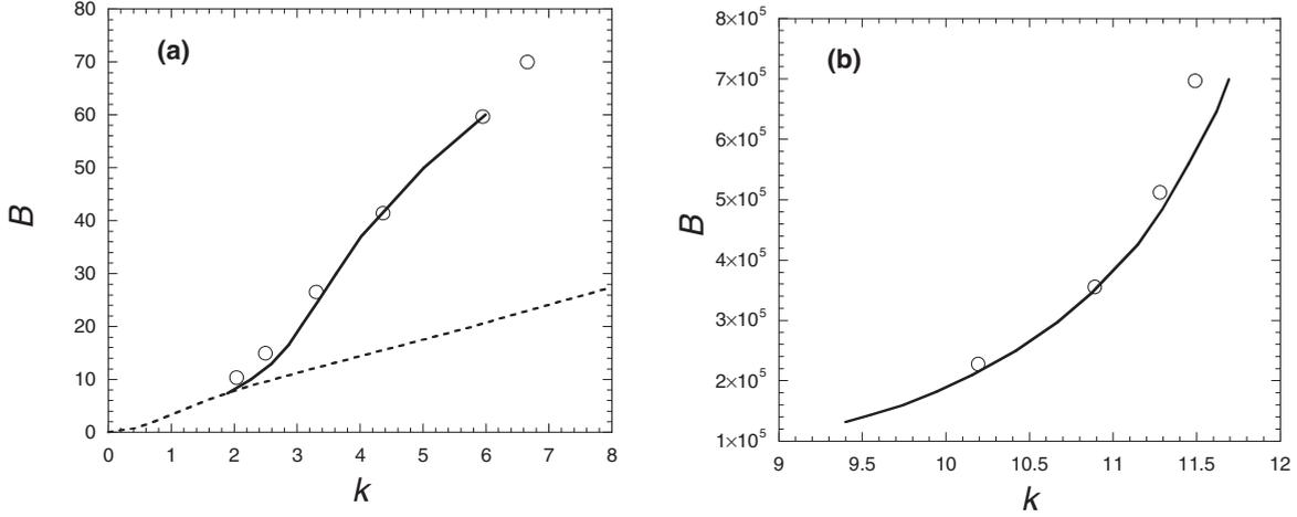
FIG. 8. Variation of the dimensionless vibrational parameter  $B$  with the dimensionless wave number  $k$  of the band pattern. Solid curve: From the numerical solution of the linearized problem of small perturbation evolution for viscous fluids [Eqs. (34)–(36)]. Circles: From direct numerical simulation. The interrupted curve is the inviscid solution Eq. (27). (a) Silicon oil and Galden HT135; (b) small surface tension and viscosity (near critical  $\text{CO}_2$  [10–12], see text).
