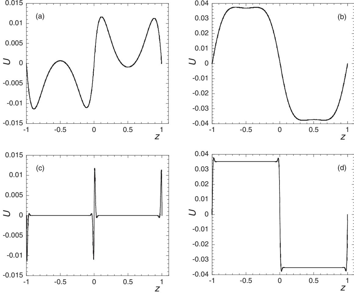
FIG. 3. Base flow velocity profiles for  $\rho_1/\rho_2 = 1.07$  and two sets of dimensionless viscosities: (a,b)  $v_1 = v_2 = 0.01$ ; (c,d)  $v_1 = v_2 = 5 \times 10^{-5}$  (typical of CO<sub>2</sub> experiments in Sec. V). Snapshots are taken at two phases of vibration period (a,c)  $\varphi = 0$  and (b,d)  $\varphi = \pi/2$ .
