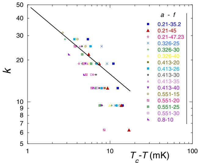
FIG. 12. Variation of the pattern reduced wave number  $k$  with respect to temperature  $T_c - T$ . Vibration parameters ( $a$ ,  $f$ ) are indicated in the figure. Full line: Power law with exponent  $-0.5$  [Eq. (38)].
