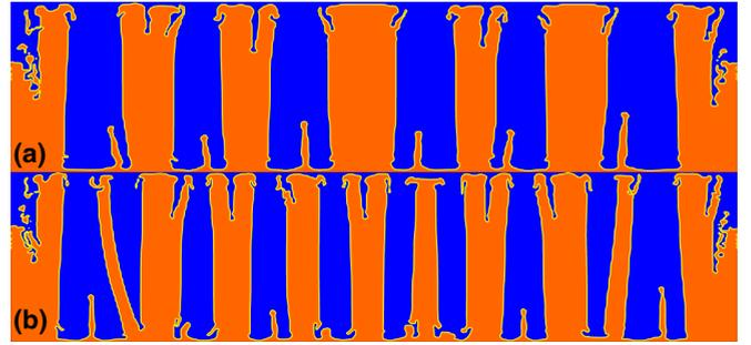
FIG. 7. Evolution of quasistationary band patterns calculated for zero surface tension with the decrease of dynamic viscosity (same for both fluids) (a)  $\eta = 0.075$  Pa.s, (b)  $\eta = 0.05$  Pa.s. Vibration characteristics are  $f = 30$  Hz,  $a = 1.8$  mm.
