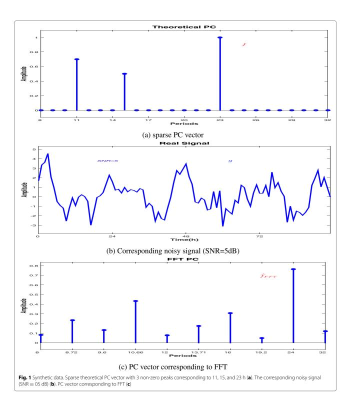
As an example, Fig. 1b presents a 4 day synthetic signal corresponding to a known PC vector (showed in Fig. 1a) and the corresponding PC vector obtained via FFT (Fig. 1c) (presented for the interval between 8 and 32 h, the circadian domain). In the synthetic PC vector,
