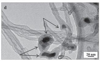
Figure 2. Transmission electron microscopy (TEM) images of multiwalled carbon nanotubes (MWCNT) dried suspensions with various concentrations of natural organic matter (NOM). (a) Without natural organic matter (MWCNT<sub>sonicated</sub>). (b) With NOM (MWCNT<sub>+NOM</sub>; ratio 1/1). (c) MWCNT<sub>+NOM</sub> (ratio 5/1). (d) Magnified view of (a). Arrows indicate metallic residues encapsulated in carbon shells or directly embedded in MWCNT.
