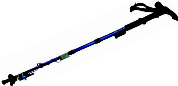
Fig. 3. Connected cane prototype equipped with a wino and its battery
