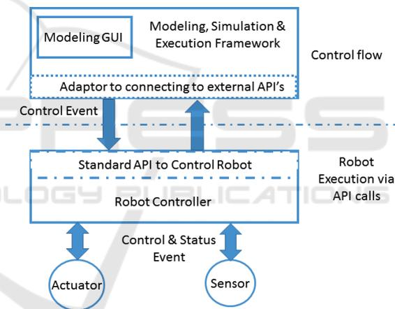
Figure 2: Conceptual Approach for Modular Complex System Development.
