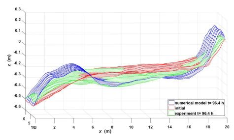
Figure 7: Three dimensional shape of the bed (bathymetry) during the second phase of simulation. Initial (red lines), numerical model (blue lines) and experiment (green lines).
