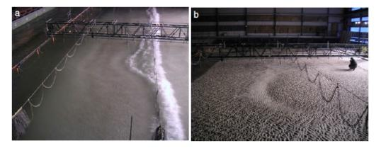
Figure 2: (a) View of a breaking wave front over the threedimensional bathymetry. Wave paddles are seen in the top left corner and the sliding beam supporting the wave gauges (1 m apart) and velocimeters are seen on top of the picture. (b) View of the emptied basin during a bathymetric survey showing the presence of a crescentic sandbar and sand ripples (Michallet et al., 2013).
