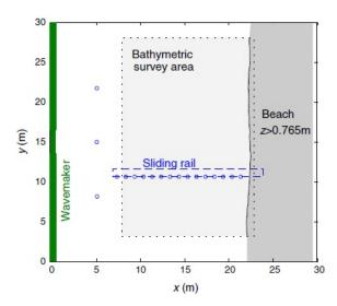
Figure 1: Schematic diagram of the basin with x and y, the cross-shore and alongshore coordinates, respectively. The mean water depth is  $h_0 = 0.765m$  for  $x \le 6m$ . The sandy beach extends from x = 6m to x = 26m. The sliding beam allows for bathymetric survey in the region shaded in grey. Circles indicate positions of the capacitance gauges (Michallet et al., 2013).
