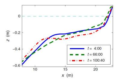
Figure 3: Alongshore-averaged beach profiles at the three main stages of the experiments (Michallet et al., 2013).
