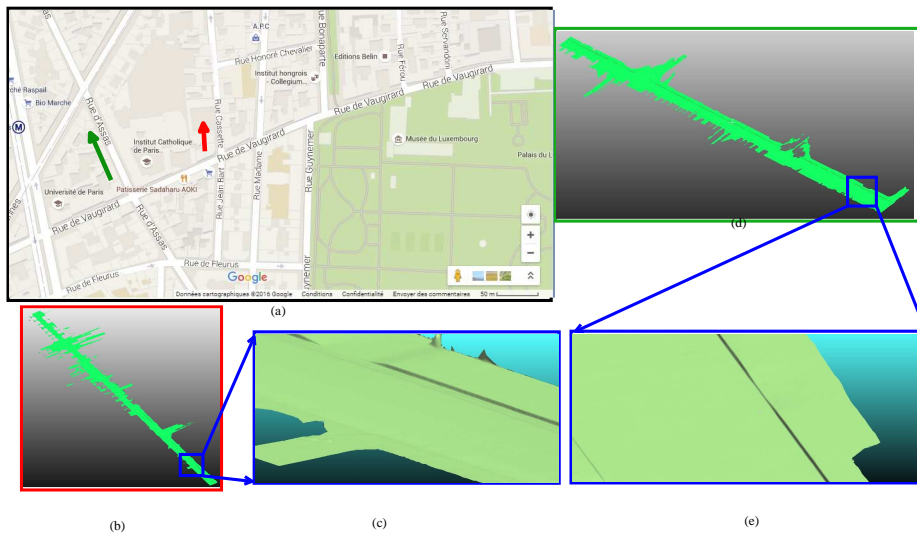
Fig. 8 Surface reconstruction results obtained for several datasets. (a) Google Maps view of two areas surveyed by the Stereopolis MMS: Assas road (Paris, France) - indicated by the green arrow, Casette road (Paris, France) - indicated by the red arrow, (b) surface reconstruction results obtained for 5 scans segments, overall length: 319 m, (c) zoom-in view of the blue rectangular area presented in Figure (b), illustrating the accuracy of the reconstructed ramp access and sidewalks, (d) surface reconstruction results obtained for 4 chunks, overall length: 217 m, (e) zoom-in view of the blue rectangular area presented in Figure (d), illustrating the accuracy of the reconstructed ramp access and sidewalks.
