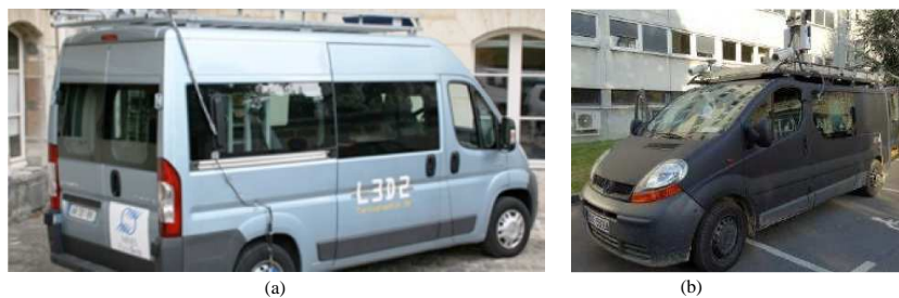
Fig. 1 Mobile mapping systems employed in the present research work: (a) L3D2 MMS prototyped by the Robotic Lab of the Mines ParisTech [30], equipped with a Velodyne 3D sensing device, (b) STEREOPOLIS prototype designed by the French Mapping Agency [29].
