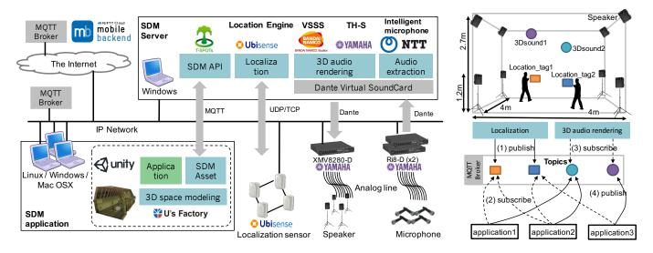
Fig. 2. Overview of SDM prototype system
