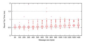
Fig. 7. RTT of MQTT messages with varying message size
