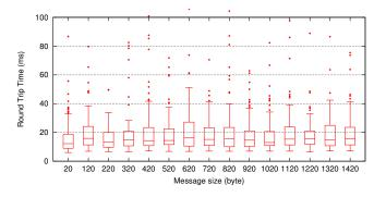
Fig. 9. RTT of MQTT messages with cloud broker
