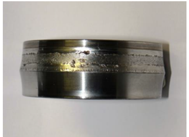
(b) Wide-spread flaking on the main bearing inner race
