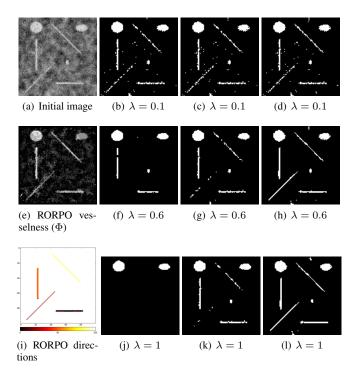
Fig. 4: Comparison of the classical Chan model (b, f, j) and the weighted TV model (c, g, k) with our directional TV model (d, h, l) for increasing regularization parameter  $\lambda$ . The direction feature is represented only inside tubular structures, in degrees, with a colormap from  $0^{\circ}$  (black) to  $180^{\circ}$  (white).
