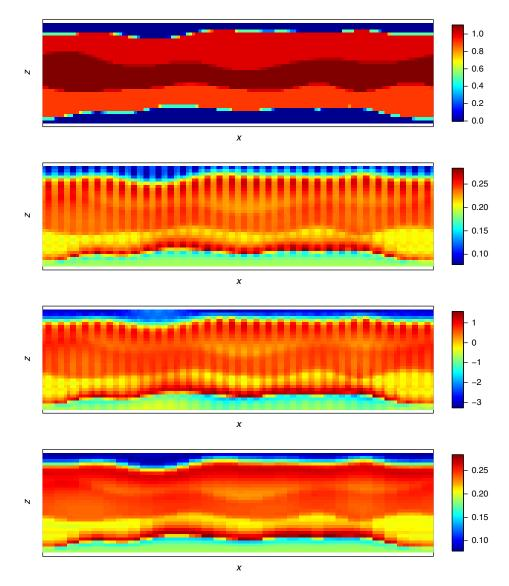
**Fig. 7** Stratigraphical phantom of dimensions  $128 \times 128 \times 32$  voxels. Plane presented: y = 22. From top to bottom: original phantom, direct inversion, inversion after normalizing values following *z*-axis, inversion after removing voxels located at edges of single reconstructions of dimensions  $4 \times 4 \times 32$  voxels.
