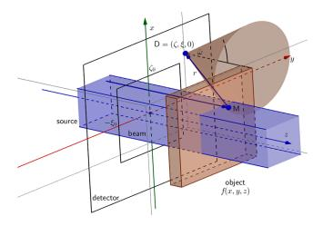
**Fig. 4** Imaging configuration proposed. A scattering site *M* produces scattered radiation captured at a detecting site *D*. The incident photon is coming from a parallel beam with a square cross-section.
