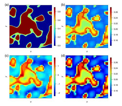
**Fig. 5** Stratigraphical phantom of dimensions  $128 \times 128 \times 32$  voxels. Plane presented: z = 4. (a) original phantom, (b) direct inversion, (c) inversion after normalizing values following *z*-axis, and (d) inversion after removing voxels located at edges of single reconstructions of dimensions  $4 \times 4 \times 32$  voxels.
