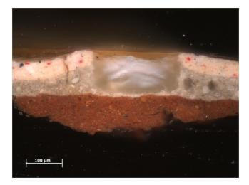
**Fig. 1** Paint cross-section showing a stratigraphical assemblage of *The Anatomy Lesson of Dr. Nicolaes Tulp*, 1632 by Rembrandt, Mauritshuis, The Hague. © Sample taken and prepared as cross-section by P. Noble during the conservation treatment of the painting in 1997 and rephotographed by A. van Loon, Mauritshuis, in 2010 for the Rembrandt Database.
