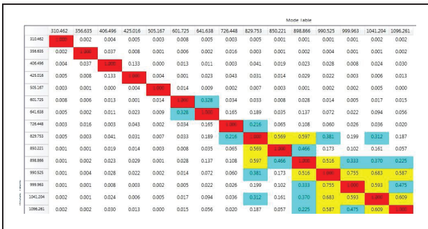
Figure 6: AutoMAC matrix for the tyre inflation pressure of 1 bar.
