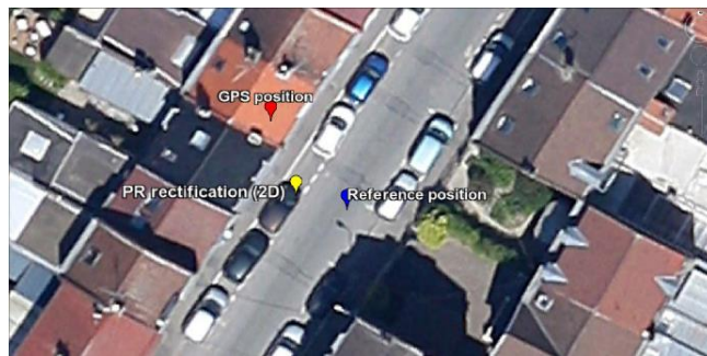
Figure 11: GPS position improvement after pseudorange correction.
