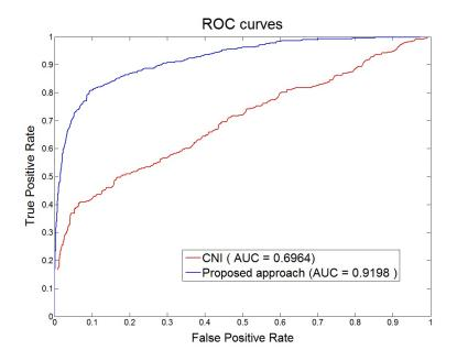
Figure. 1. Receiver operating characteristic (ROC) curve for the proposed method (blue) and for the standard CNI approach (red).
