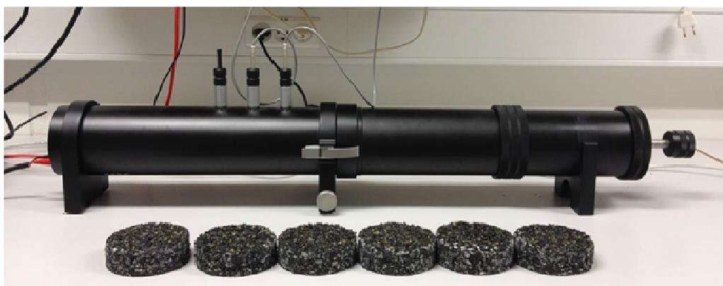
Figure 10 - Impedance tube for measuring acoustical absorption.
