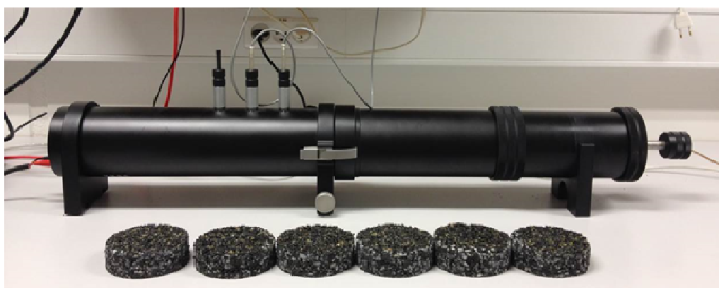
Figure 10 - Impedance tube for measuring acoustical absorption.
