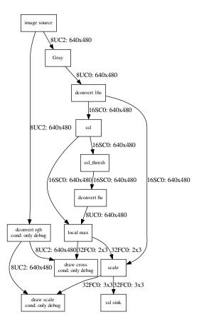
Figure 1: Example of processing tree for the extraction of Self-Similar Landmarks
