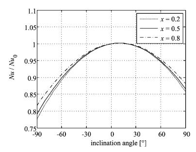
Fig. 20. Effect of the inclination angle on the heat transfer for R134a condensing in a microfin 8.92 mm inside diameter tube at mass fluxes from 54 to  $107 \text{ kg/m}^2\text{s}$  (Akhavan-Behabadi et al., 2007).
