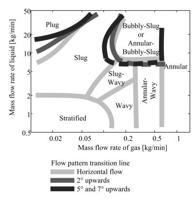
Fig. 11. Effect of the inclination angle on a flow pattern map (Ghajar and Kim, 2005).
