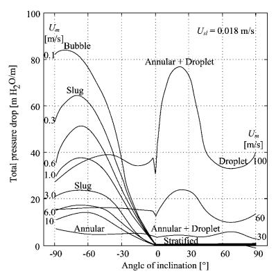
Fig. 15. Pressure drop as a function of the inclination angle, adapted from Spedding et al. (1982) (air-water flow in a 4.55 mm inner diameter pipe;  $U_{\rm sl}=0.018$  m/s).
