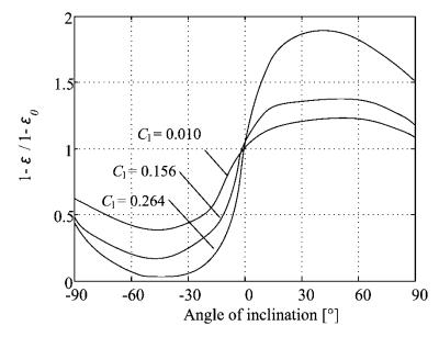
Fig. 12. Inclination correction angle as a function of inclination angle, adapted from Beggs and Brill (1973).
