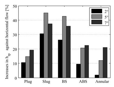
**Fig. 16.** Effect of the inclination angle on the heat transfer coefficient (BS: Bubbly-Slug, ABS: Annular-Bubbly-Slug), adapted from Ghajar and Kim (2005).
