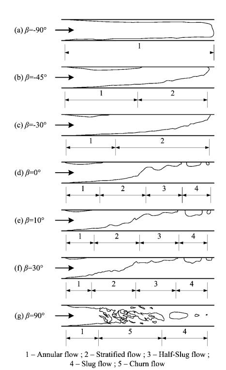
**Fig. 19.** Schematic drawings of condensation flow patterns for orientations, adapted from Wang et al. (1998).
