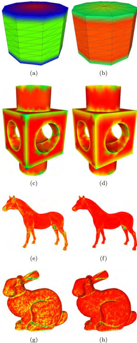
Figure 8: *Prism*, *Block*, *Horse* and *Bunny* meshes colored according to the Hausdorff distance after a cycle of transformations. 1) Left, subfigures a), c), e) and g) using *Center of Mass*. 2) Right, subfigures b), d), f) and h) using our method based on *Distance to the tangent planes*.
