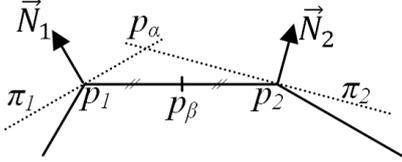
Figure 3: Solution of equation (6) as the affine combination of the generalized intersection of planes  $\pi_i$  ( $p_\alpha$ ) and the average of all points  $p_i$  ( $p_\beta$ , for  $\beta_i = \beta$ ).
