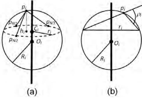
Figure 2: a) Tetrahedron formed by point  $p_i$  and its 3 neighbors  $p_{N1(i)}, p_{N2(i)}, p_{N3(i)}$ , with the circle defined by the neighbors, and the sphere containing those four points. b) Projection on a plane passing through  $O_i, C_i$  and  $p_i$ , revealing the simplex angle.
