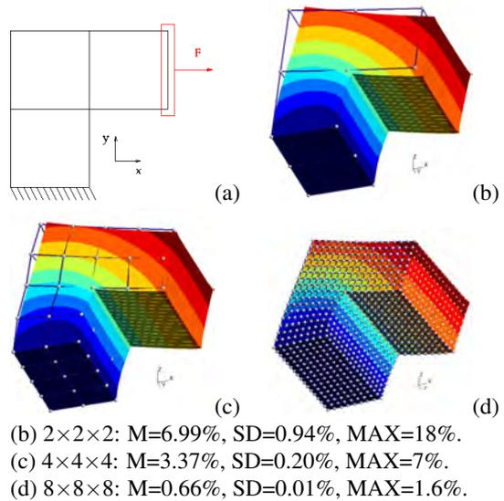
**Figure 6:** Experiment on a non-symmetric object: (a) load scheme, (b-d) the reference FEM solution (in color gradation) with superimposition of various simulations performed for different mesh resolutions.
