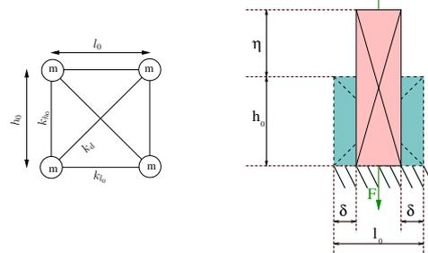
**Figure 1:** (Left) 2D rectangular element with three pairs of strings:  $k_{l_0}$ ,  $k_{h_0}$  and  $k_d$ . (Right) The bar is elongated by a force  $\vec{F}$ , generating a stretch  $\eta$  and a compression of  $2\delta$  at equilibrium.
