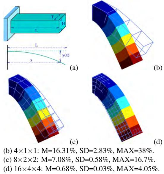
**Figure 5:** Deflection experiment: (a) Cantilever neutral axis deviation, (b-d) the reference FEM solution (in color gradation) with superimposition of various simulations performed for different sampling resolutions (wire mesh).
