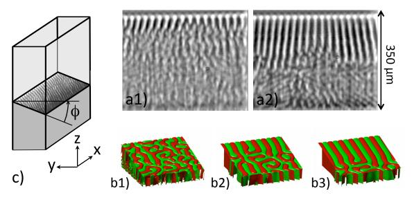
Figure 4. Real-time observations: a1) and a2) Global drift of a labyrinth pattern and formation of regular lamellae by an invasion process due to a thermal-bias effect. b1) to b3): Phase field simulations of this morphological transition at three successive instants (thermal-bias angle  $\phi = 12^{\circ}$ ). c) Schematic representation of the thermal bias.
