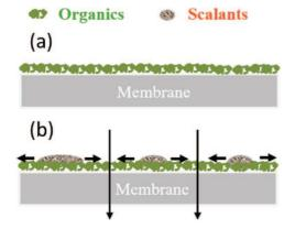
Fig. 12. Foulants on the membrane surface (a) without and (b) in presence of scaling.
