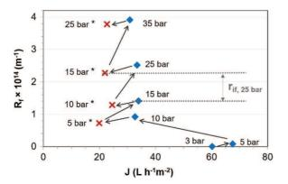
**Fig. 6.** Evolution of the total fouling resistance  $(R_f)$  v.s. pseudo stable flux obtained at each pressure according to the square-wave method procedure.  $R_f$  after a positive variation of pressure  $\blacklozenge$ ;  $R_f$  after a negative variation of pressure  $\bigstar$ . Arrows represent the variations of pressure during the procedure.
