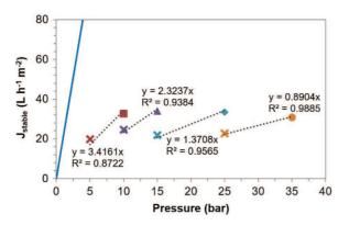
**Fig. 13.** Experimental permeability measurement, the continuous line - is initial permeability of membrane; bold points are the first pseudo stable fluxes reached at a certain pressure; the crosses are the stable fluxes reached after negative variation of pressure (5 bar\*, 10 bar\*, 15 bar\*, 25 bar\* in Fig. 4).
