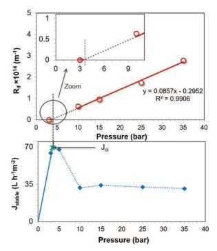
**Fig.** 7. Evolution of (a) irreversible fouling resistance, (b) pseudo stable flux as function of pressure and the location of the critical flux for irreversibility  $\mathbf{x}$ .
