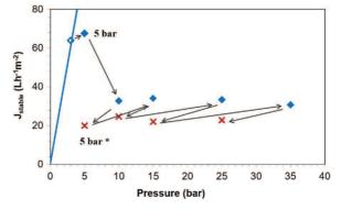
Fig. 5. Pseudo stable flux vs applied pressure following the procedure shown on Fig. 3; initial permeability \_\_\_\_\_\_\_; first pseudo stable flux reached at a certain pressure ♦: hollow one is without decrease of flux over time and the bold points are in presence of flux decrease during filtration; stable flux reached after negative variation of pressure **X** (5 bar\*, 10 bar\*, 15 bar\*, 25 bar\* in Fig. 3); Arrows represent the positive or negative variations of pressure.
