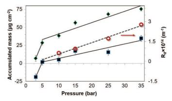
**Fig. 11.** Evolution of irreversible fouling resistance  $\bigcirc$  and ions accumulated mass: Ca<sup>2+</sup>  $\blacksquare$ , PO<sub>4</sub><sup>3-</sup>  $\blacklozenge$  on the membrane with increasing applied pressure during recirculation step.
