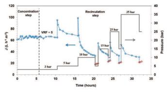
**Fig. 4.** Flux evolution following the experimental procedure over time: – the continuous line represents the applied pressure; the dotted line denotes the permeate flux.
