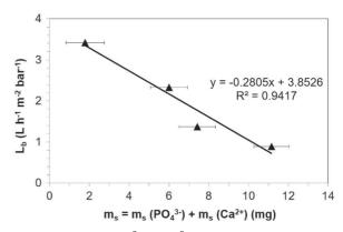
Fig. 14. Relationship between  $Ca^{2+}$  and  $PO_4^{3-}$  accumulated mass on membrane and  $L_b$  permeability combining two fouling mechanisms.
