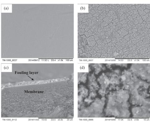
Fig. 10. SEM images of virgin and fouled membrane: (a) Clean membrane surface 1000×; (b) Fouled membrane surface 1000×; (c)Section of fouled membrane 5000×; (d) Fouled membrane surface 10000×.
