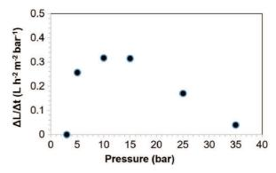
Fig. 8. Permeability loss rate obtained at different pressure values.
