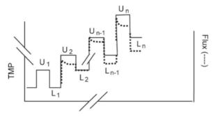
Fig. 2. Principle of the square-wave technique; pressure and flux vs time; upper and lower steps [5].
