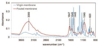
Fig. 9. ATR-FTIR spectra of fouled and clean membrane.
