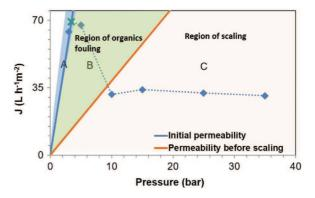
**Fig. 15.** Experimental pseudo stable flux as a function of transmembrane pressure and the location of the critical flux for irreversibility **x** in working diagram of NF considering the initial permeability and the permeability before scaling.
