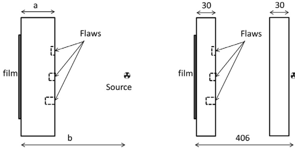
**Fig. 4:** First case study involves two simple wall configurations (left), with  $a = 92$  mm and  $b = 390$  mm (respectively  $a = 56$  mm and  $b = 421$  mm) and one double wall configuration (right).
