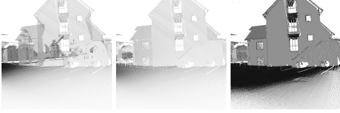
(a) Point cloud projection (b) Occlusion estimation (c) Interpolation
