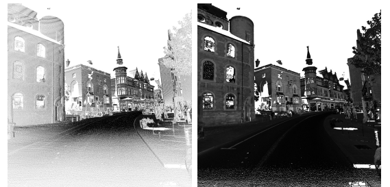
(a) No interpolation (b) Bilinear interpolation
