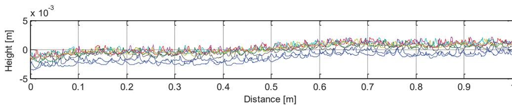
Figure 14 – Examples of longitudinal profiles extracted from the enveloped surface
