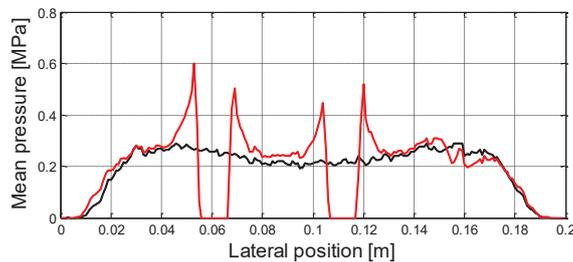
Figure 13 – Contact pressure averaged over the rolling direction - Red curve: patterned E3A tyre – Black curve: slick tyre
