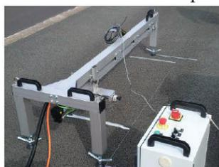
Figure 2 – 3D texture measurement system
