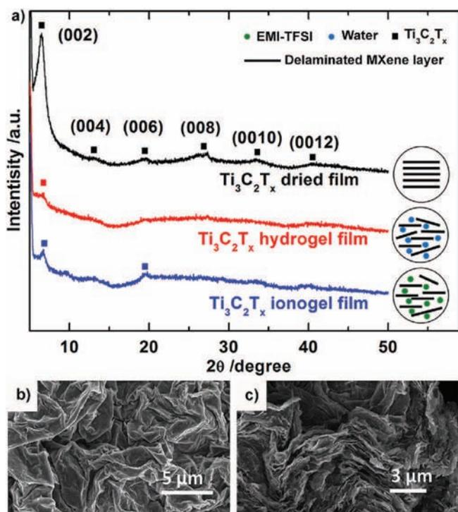
**Fig. 2.** a) XRD patterns of  $\text{Ti}_3\text{C}_2\text{T}_x$  dried film, hydrogel film and ionogel film; b, c) SEM images of  $\text{Ti}_3\text{C}_2\text{T}_x$  ionogel film: b) top view; c) cross-sectional view.
