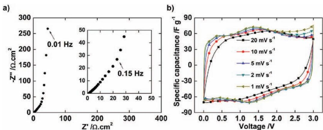
Fig. 5. Electrochemical characterization of thick Ti<sub>3</sub>C<sub>2</sub>T<sub>x</sub> ionogel film with mass loading of 4 mg cm<sup>-2</sup> (mass of Ti<sub>3</sub>C<sub>2</sub>T<sub>x</sub> only): a) Nyquist plot of 2-electrode Swagelok cell; b) CVs of 2-electrode Swagelok cell with voltage window of 3 V.
