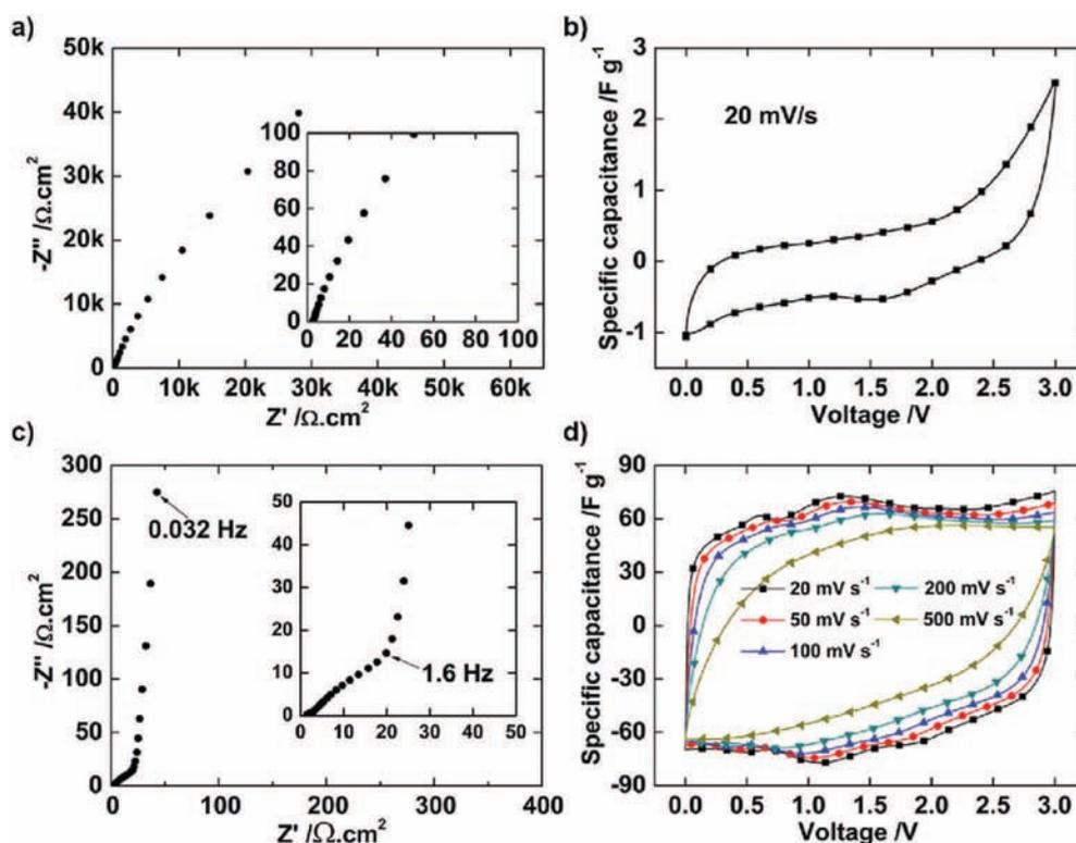
**Fig. 3.** a) Nyquist plot and b) CV of  $\text{Ti}_3\text{C}_2\text{T}_x$  dried film tested in EMI-TFSI ionic liquid electrolyte. Electrochemical characterizations of  $\text{Ti}_3\text{C}_2\text{T}_x$  ionogel film with mass loading of  $0.76 \text{ mg cm}^{-2}$  (mass of  $\text{Ti}_3\text{C}_2\text{T}_x$  only): c) Nyquist plot of a 2-electrode Swagelok cell; d), CVs of a 2-electrode Swagelok cell at scan rate from 20 to  $500 \text{ mV s}^{-1}$  within a voltage window of 3 V.
