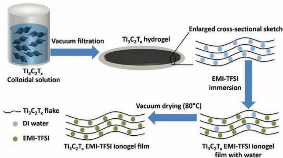
Fig. 1. Schematic of producing  $\text{Ti}_3\text{C}_2\text{T}_x$  EMI-TFSI ionogel film.
