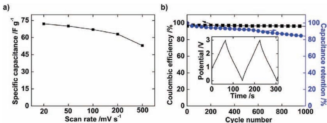
Fig. 4. a) Change of the specific capacitance with scan rate; b) Capacitance retention test of Ti<sub>3</sub>C<sub>2</sub>T<sub>x</sub> film at 1 A g<sup>-1</sup> and coulombic efficiency of 2-electrode Swagelok cell.
