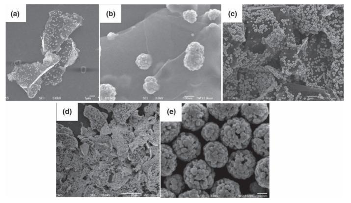
Fig. 1. SEM images of  $Fe_{3-x}O_4$ /graphene sheets nanocomposites with different weight ratios  $Fe_{3-x}O_4$ /graphene: NC-100 (a,b), NC-20 (c) and NC-10 (d) and of isolated nanostructures showing  $Fe_{3-x}O_4$  aggregates constituted by assembly of several nanocrystals (e).
