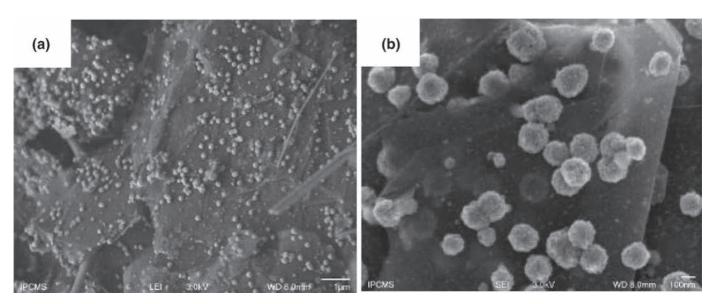
Fig. 8. SEM images of the raspberry nanostructures after 50 charge/discharge cycles showing the high stability of the iron oxide aggregates after charge/discharge cycles. Some sintering is observed as indicated by arrows.
