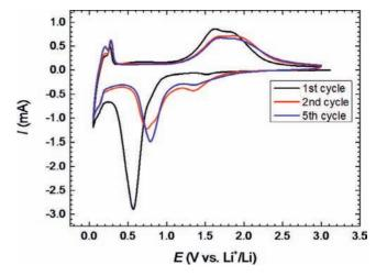
Fig. 5. Cyclic voltammograms of the  $Fe_3O_4$  raspberry/graphene sheets in 1 M LiPF<sub>6</sub> in EC: DMC (1: 1 in volume ratio) electrolyte, at 0.2 mV/s.
