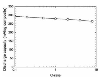
Fig. 7. Power plot for the  $Fe_3O_4$  raspberry/graphene sheets containing 50 wt% of  $Fe_3O_4$ ; details of the power plot construction is given in experimental section.
