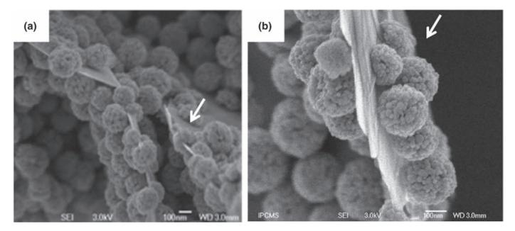
Fig. 2. High resolution SEM micrographs of the nanostructure/FLG composite showing the anchorage of the iron oxide aggregates on both side of the graphene sheet and also the presence of strong oxide/support interaction leading to the formation of iron oxide hemispheres aggregates (indicated by arrows).
