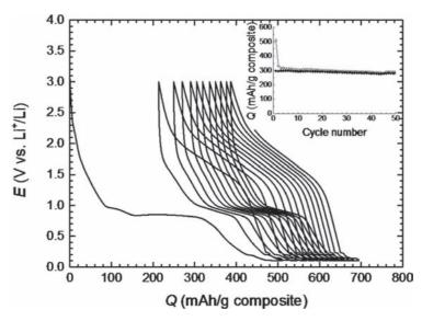
Fig. 6. Galvanostatic charge/discharge plots for the Fe<sub>3-x</sub>O<sub>4</sub> nanostructures/graphene sheets containing 50 wt% of Fe<sub>3-x</sub>O<sub>4</sub>, at 1 C rate.
