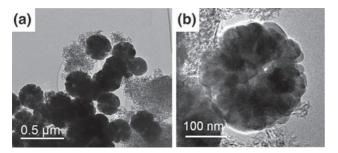
Fig. 3. TEM analysis of the  $Fe_{3-x}O_4$  nanostructures showing the presence of  $Fe_{3-x}O_4$  nanoparticles with diameter ranged between 30 mm and 70 nm within the aggregate.
