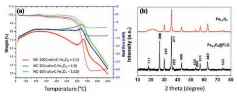
Fig. 4. (a) TG-DTA curves of NC-100, NC-20 and NC-10 and (b) XRD pattern of NC-10 (This XRD pattern is characteristic of those of all composites).
