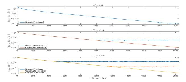
**Figure 2.** Decay of the FOURIER coefficients for  $\varepsilon = 0.4$  and  $kd = \infty$ . Blue: 16 digits; Red: 34 digits; Orange: 71 digits.
