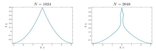
**Figure 1.** Influence of the number of FOURIER modes for  $kd = \infty$ ,  $\varepsilon = 0.4401$ . Left: normal solution obtained with N = 1024. Right: ghost solution obtained with N = 2048.
