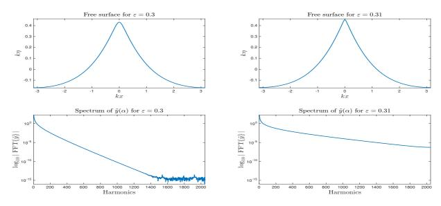
**Figure 3.** Examples of steep waves in finite depth for kd = 1. Left:  $\varepsilon = 0.3$ ; Right:  $\varepsilon = 0.31$ ; Upper: free surfaces; Lower: spectra.
