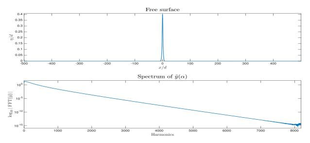
**Figure 4.** Cnoidal wave in very shallow water (L/d = 1000, H/d = 0.4).
