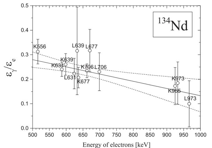
FIG. 3. The efficiency curve ( $\epsilon_\gamma/\epsilon_e$ ) of the experimental setup for the  $^{134}\text{Nd}$  measurement. The linear fit to the experimental points and the error band are indicated by solid and dashed lines, respectively.
