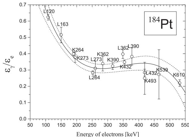
FIG. 7. The efficiency curve ( $\epsilon_\gamma/\epsilon_e$ ) vs electron energy for the experimental setup ( $^{184}\text{Pt}$  experiment). The third-order polynomial fit to the experimental points and the error band are denoted by solid and dashed lines, respectively.
