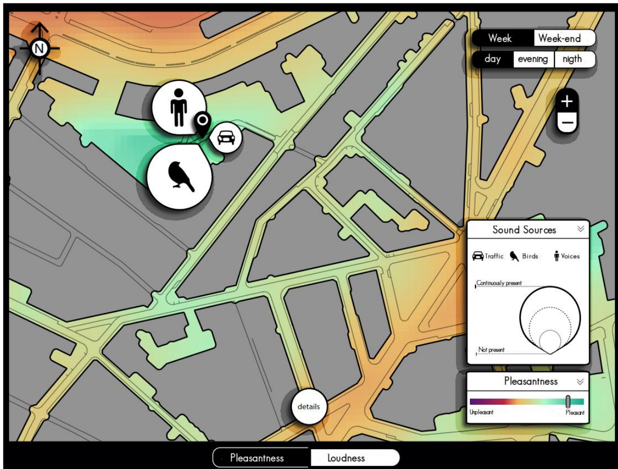
Figure 19: Final representation of the sound quality with visualization of sound source presence and visualization of the period of the selected map (buttons in black).
